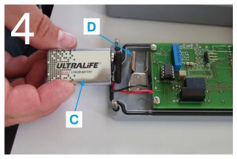
Remove the battery (C) carefully out of its fixture (D).
