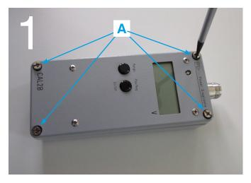
Release the four screws (A) in the corners of the calibrator's front.
