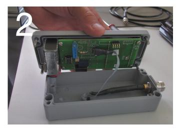
Open the calibrator's enclosure carefully.
