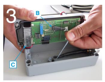
Disconnect the four pin connector (B) of the calibrator's output by slightly pulling it.
