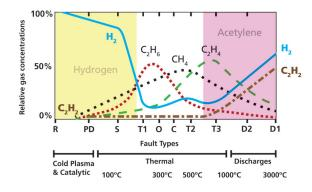
The graph above shows the value of hydrogen  $(H_2)$  in detecting the early phases of a fault as well as the critical value of acetylene  $(C_2H_2)$  if and when the fault progresses to a level which requires immediate attention.
