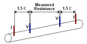
To ensure a uniform current density through a bar, the potential leads should be separated from the current leads by at least a distance of 3 times the width of the sample being measured.
