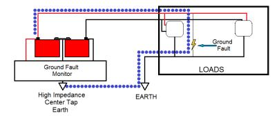
If a second ground fault occurs, this creates another path for current. Depending on the location and impedance of this ground fault, significant current can be drawn. This can cause a relay to trip taking a critical system off line, damaging equipment or injuring personnel.
