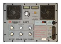
The BGFT has a built in Wheatstone bridge which allows the user to determine the actual capacitance and resistance on the circuits. This ensures that no time is wasted tracing a false path. The BGFT allows the circuit to be identified with the fault.
