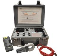
The BGFT has two output ranges. The low voltage range is specifically designed not to trip breakers even under conditions of misuse. In addition the BGFT injects a low frequency, low current AC signal between the side of the battery that is faulted and earthed.
