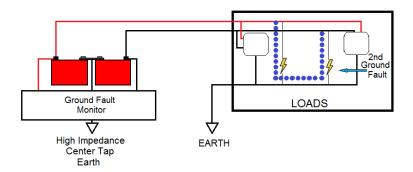
However, knowing a ground fault exists and locating it are two different issues. To locate a ground fault, a pulsed or AC current is injected between the side of the battery string and earth that will follow the path of the ground fault. By tracing the path of this current the ground fault can be located. However, there are several risks that need to be avoided when tracing a ground fault. These include the following:
