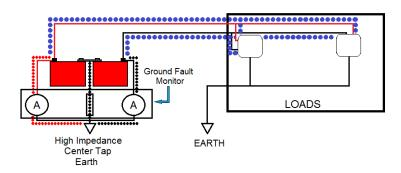
When there is no ground fault, the current through the positive and negative paths of the ground fault monitor are equal. In the presence of a ground fault, the currents become unbalanced in the ground fault monitor and a ground fault will be detected. This will also create an unbalance in the voltages between positive the terminal to earth and negative terminal to earth.
