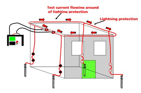
As can be seen in the above diagram, none of the test current flows through the earth mass. In fact the measurement will be a short circuit.
