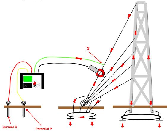
The error isn't at first obvious, I want to measure the earth resistance of the guy line with the clamp around it. But the guy lines on this tower are all shorted together. The current being measured by **ICLAMP** is flowing not just to ground at the anchor point, but back up the other guy lines and to ground via the tower. This means the calculated resistance will be incorrect for the anchor point.
