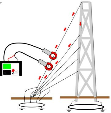
As the guy line are all linked together both at the tower metal work and at the anchor point, a loop is formed, and no current flows through the earth mass. Hence the reading will not be the resistance of the guy line to earth.
