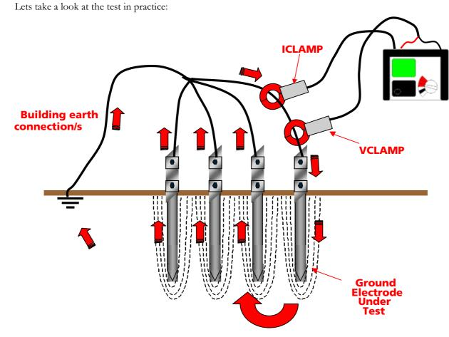
Current is induced into the circuit by the **ICLAMP** and then the resulting voltage is measured with the
