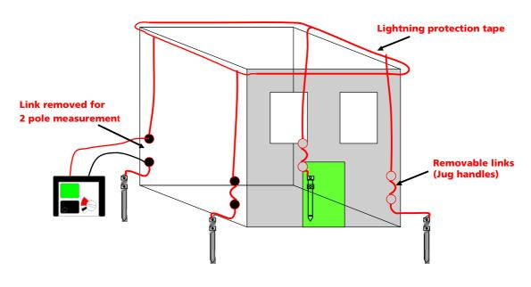
Using the stakeless method negates the requirement to remove these links, just clamp the **ICLAMP** and **VCLAMP** around the tape or link. See below
