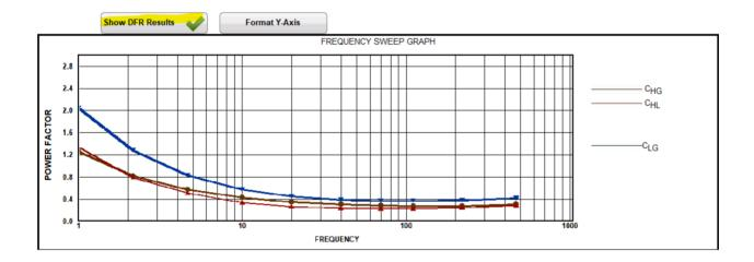
The superior sensitivity of 1 Hz PF/DF detects insulation changes well before PF/DF measured at power frequency does. Combined with a 10 kV traditional PF/DF instrument, 1 Hz PF/DF provides the means to immediately validate line frequency PF/DF results.
