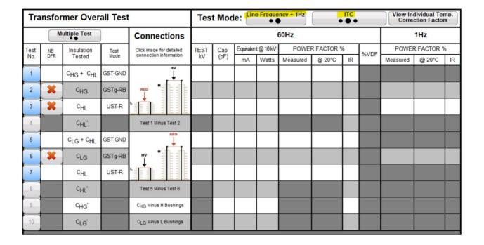
After completing the test, PowerDB automatically provides a colour-coded condition assessment of the insulation for tests performed at power frequency and 1 Hz. The table below displays the 'traffic light' assessment values for power frequency and 1 Hz temperature-corrected, % PF/DF test results:
