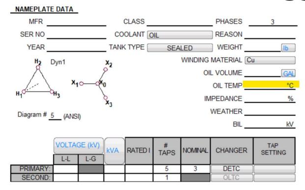
PowerDB forms for the DELTA4000 are preconfigured to measure 1 Hz PF/DF using the same test connections as those for the power frequency PF/DF measurement. First, select the type of test you want to perform.
